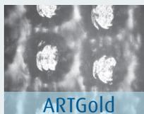
*ARTGold* imprints using the Anilox Reverse Technology (ART), raising "pins" between the cells. Initially designed for flexographic printing, it has become a standard for offset coating and for laying water-based and UV adhesives and coatings. It is perfect for high opacity white ink.
