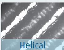
The Helical engravings open structure offers a much better release for the gravure and coater applications. Optimizes the use high viscosity materials, and high volume capacity operations.
