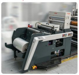
New concept with independent motor on the reel. Expandable shaft, supported on both side, with automatic lifting device for effortless reel changeover operations. A dedicated reel trolley from pallet to unwinder is available to help the operator in daily operations.
